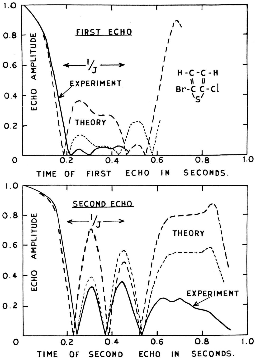
2. Echo amplitude modulation from multiple shot experiments in 2-bromo-5-chlorothiophene at 25° C, (a) the first echo and (b) the second echo of a  $90^\circ, \tau, 180^\circ, \tau, \text{Echo}_1, \tau, 180^\circ, \tau, \text{Echo}_2$  sequence. The theoretical curves are for  $\delta = 3.97$  c/s and  $J = 3.87$  c/s without attenuation.
