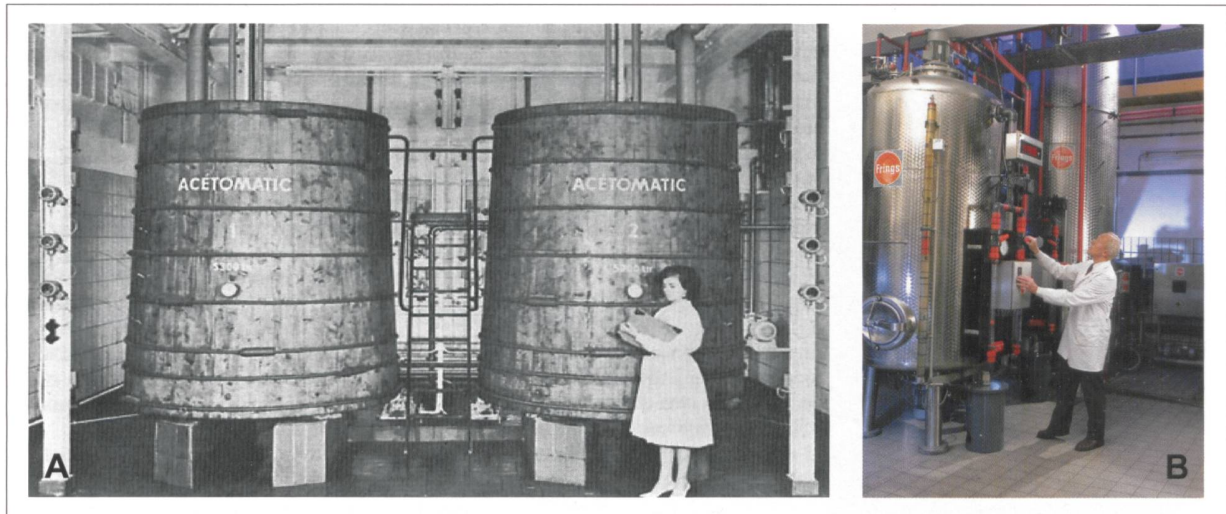
Fig. 10: Submerged acetification systems.
