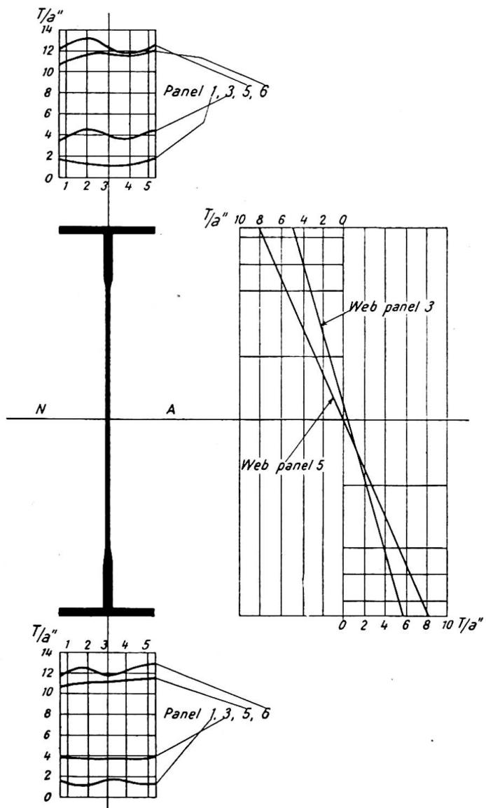
**Fig. 4.** Tests on model girder bending stresses in flanges and web load 75 tons
