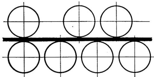
Fig. 1. Arrangement of rolls. Roller levelling machine
