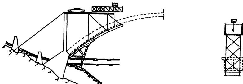
FIG. 1. Formwork for a 112 m concrete arch
