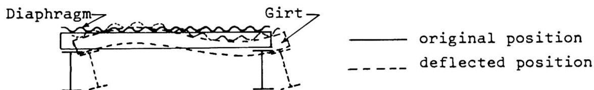
Fig. 4 Columns with Diaphragm-Girt Bracing
