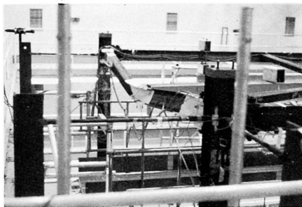
Fig. 5 - Major-Axis Beam at Collapse
