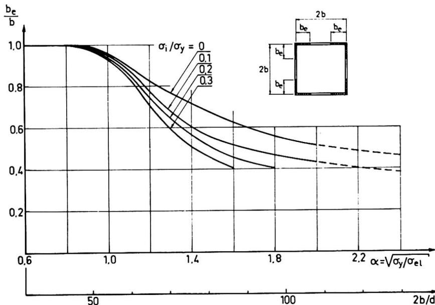
Fig. 3 Ratio  $b_e/b$  for the failure load as a function of  $\alpha$
