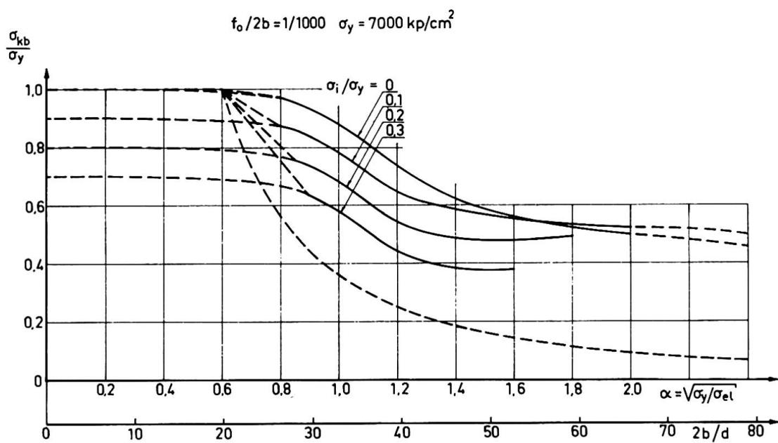
Fig. 2 a and 2 b. Values of  $\sigma_{kb} = N/2bd$  at buckling failure divided with  $\sigma_y$  for different  $\sigma_i/\sigma_y$  as function of  $\alpha = \sqrt{\sigma_y/\sigma_{el}}$
