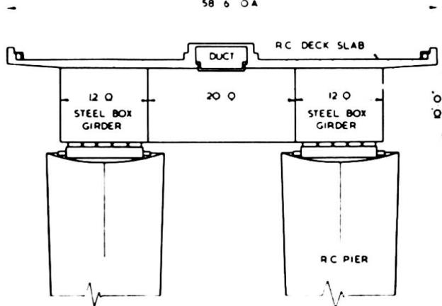
FIG. 1 TYPICAL CROSS SECTION.
