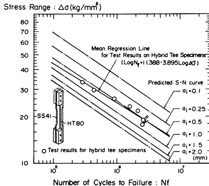
Fig.4 Comparison of Predicted S-N Curves and Previous Fatigue Test Results on Hybrid Tee-shaped Specimen(1)
