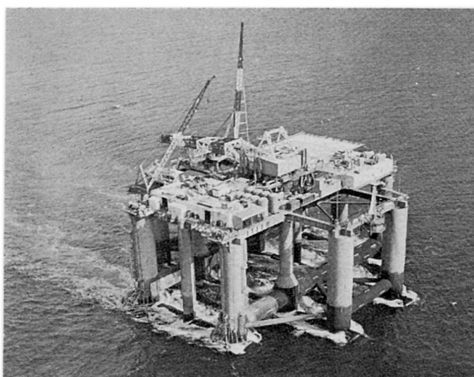
Fig. 10. Self-propelled multiple-hull Semi-submersible
