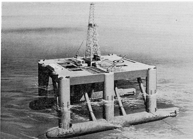
Fig. 6. Twin-hull Self-propelled Semi-submersible
