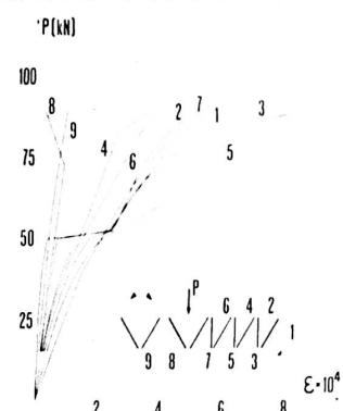
STRAINS IN VERTICAL RODS AND DIAGONALS
