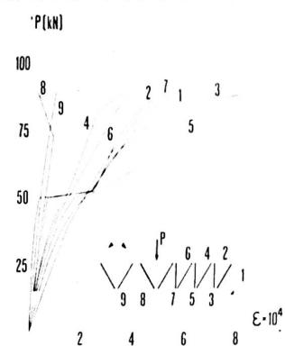
STRAINS IN VERTICAL RODS AND DIAGONALS
