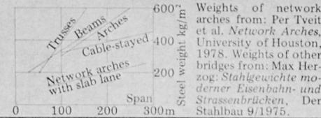
Weights of network arches from: Per Tveit et al. *Network Arches*, University of Houston, 1978. Weights of other bridges from: Max Herzog: *Stahlgewichte moderner Eisenbahn- und Strassenbrücken*, Der Stahlbau 9/1975.
