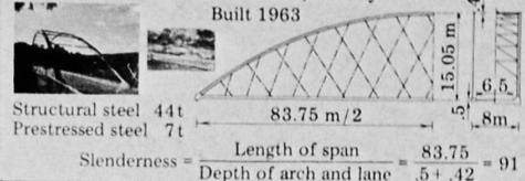
When many hangers relax bending moments in the chords are bigger than when the span acts like a truss. The normal forces in the chords, however, are smaller than maximum because the live load is only on part of the span.
