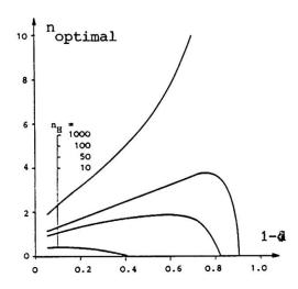
Figure 1: Optimal number of control checks versus control efficiency
