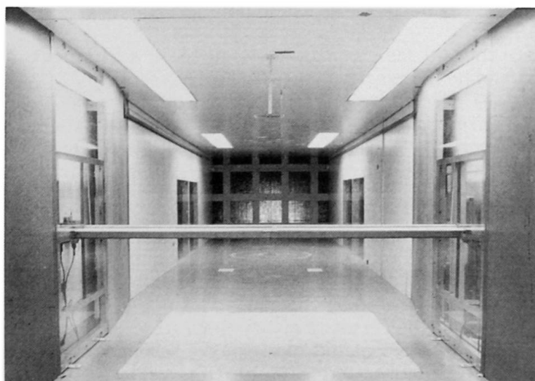
Fig. 5 Section Model in Wind Tunnel
