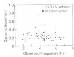
Dynamic load allowance is a fraction of highway live load to cater for dynamic effects of vehicle & bridge, and riding surface irregularity.
