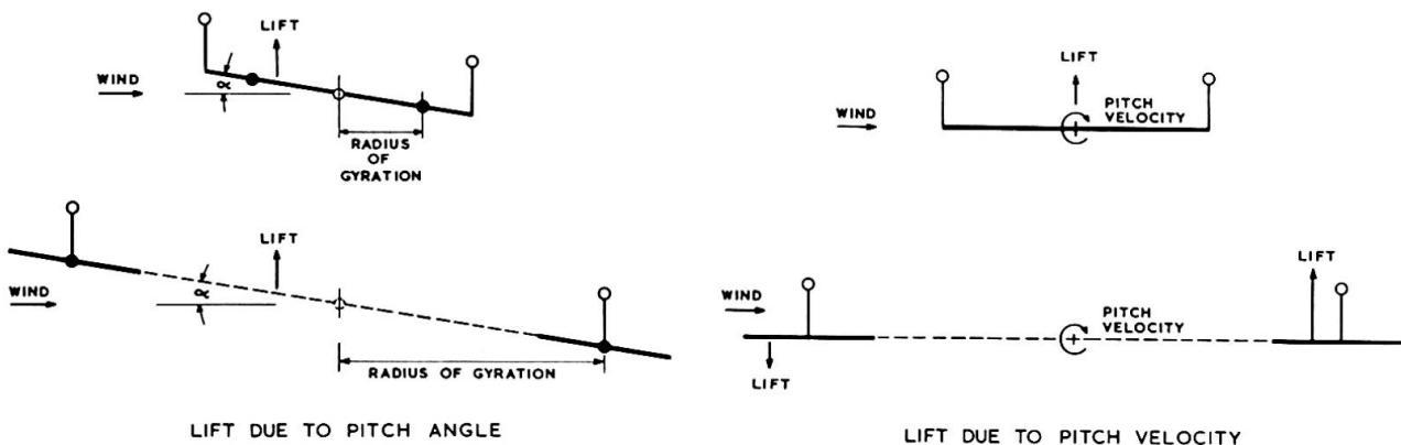
Torsional stiffness can be achieved, without weight penalty, by spacing the cables much further apart. If at the same time, the two deck halves are also separated to hang directly under each cable leaving a huge "slot" between them, three phenomena occur. With the understanding that the two decks are constrained to move as a single body by rigid transverse beams at intervals along the span, then
