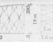
$$\frac{\Sigma 128 \text{ t}}{7 \times 100} = 183 \text{ t/m}^2 \quad \text{Slenderness } \frac{100}{.395 + .3} = 144$$
