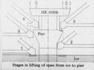
Stages in lifting of span from ice to pier
