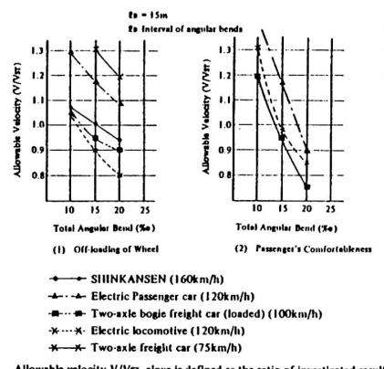
Allowable velocity  $V/V_{st}$  slope is defined as the ratio of investigated result to standard running speed
