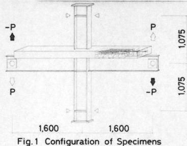
Fig. 1 Configuration of Specimens
