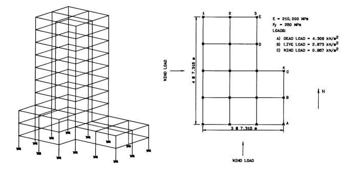
Fig. 4 a) Simplified isometric view of example structure, b) Dimension, material properties, and specified loads.
