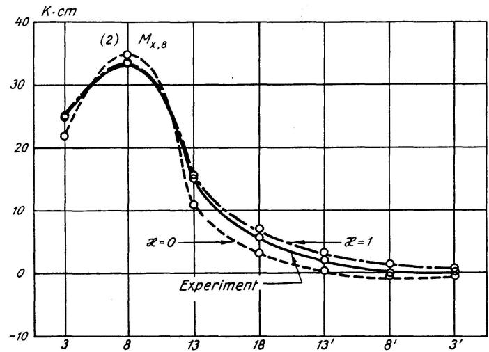
Fig. 11. Comparison of the Bending Moments Calculated from the Measured Strain Gauge Readings and from the Theory for the Model c)<sub>2</sub> ( $A = 4$ ,  $B = 0.5$ ).
