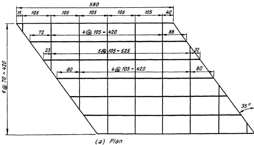
Fig. 7. The Plan of the Skew Grillage Girder Bridge ( $A = 1$ ,  $B = 0.5$ ) and the Cross Section of the Main and Cross Girders.
