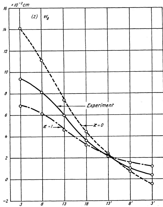
Fig. 9. Comparison of the Deflections Calculated from the Measured Dial Gauge Readings and from the Theory for the Model c<sub>1</sub> ( $A = 1$ ,  $B = 0.5$ ).
