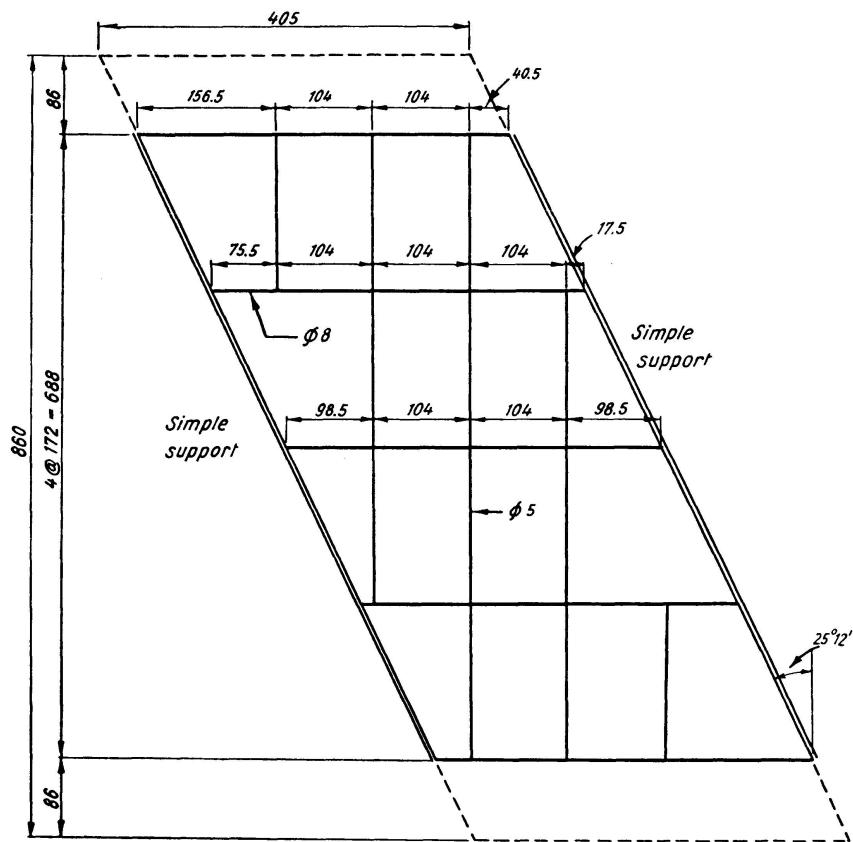
Fig. 5. The Plan of the Skew Grillage Girder ( $A = 9$ ,  $B = 1$ ).
