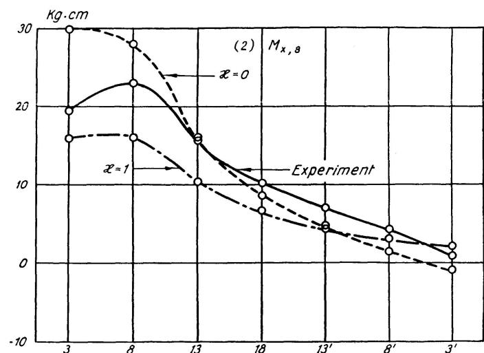
Fig. 10. Comparison of the Bending Moments Calculated from the Measured Strain Gauge Readings and from the Theory for the Model c)<sub>1</sub> ( $A = 1$ ,  $B = 0.5$ ).
