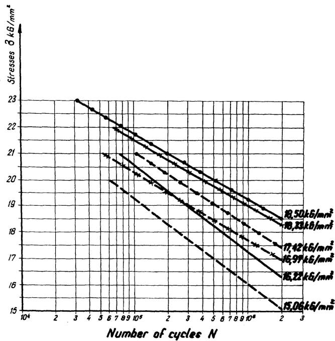
Fig. 3. Wöhler's diagrams for the coefficient  $\kappa = 0$ .
