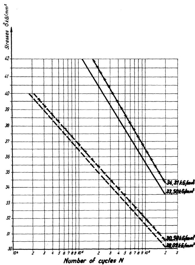
Fig. 2. Wöhler's diagrams for the coefficient  $\kappa = 1,25$ .
