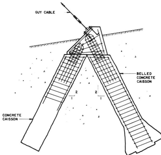
Fig. 2 Tension anchor
