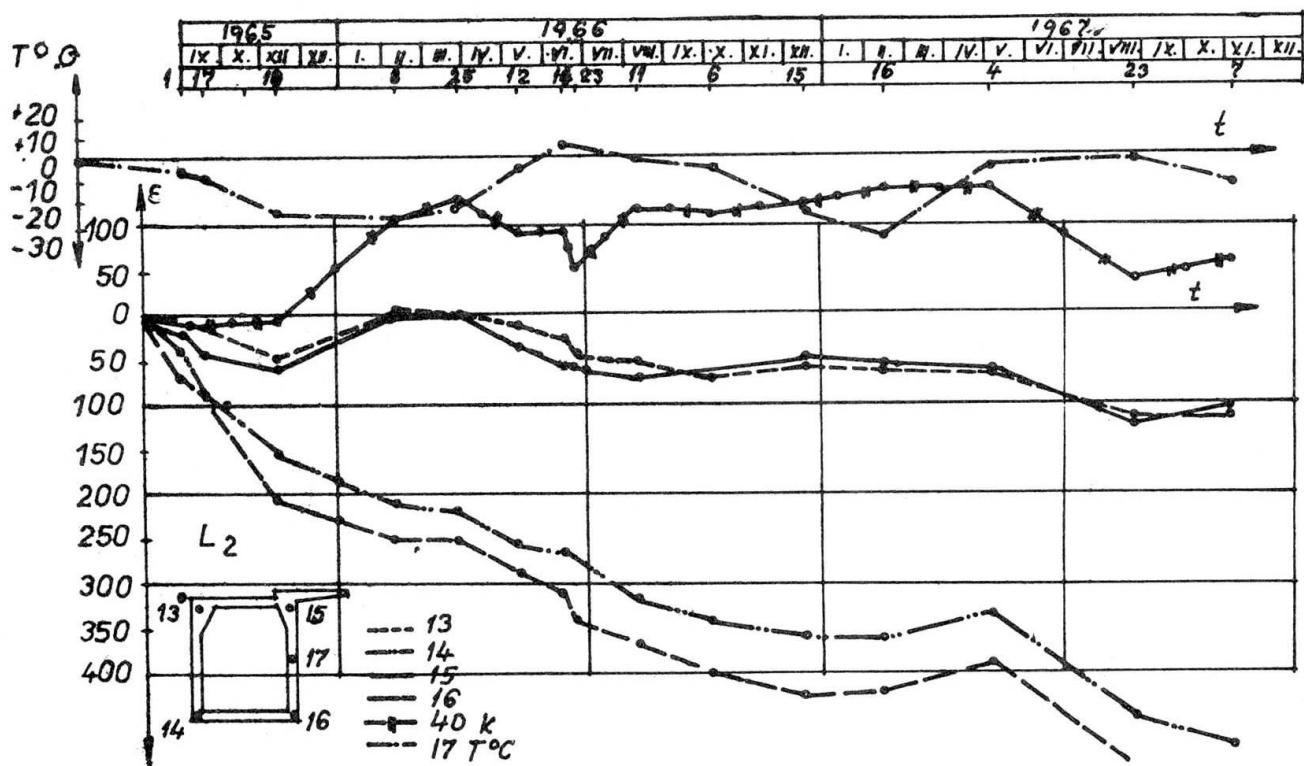
Fig.No.6.: The strains  $\epsilon \times 10^{-6}$  in the cross section at the fixed end (first precast element) of the cantilever highway bridge " S " with prestressed concrete precast elements during the first 2 years.
