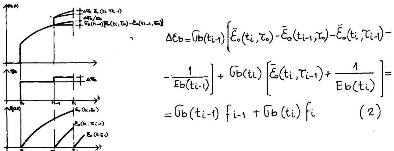
FIG. 3 FINITE VARIATION OF CREEP STRAIN
