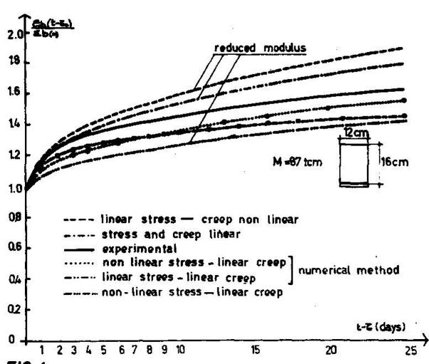
FIG. 4 COMPARISON OF THEORETICAL AND EXPERIMENTAL DEFORMATION RATIOS OF REINFORCED CONCRETE BEAM
