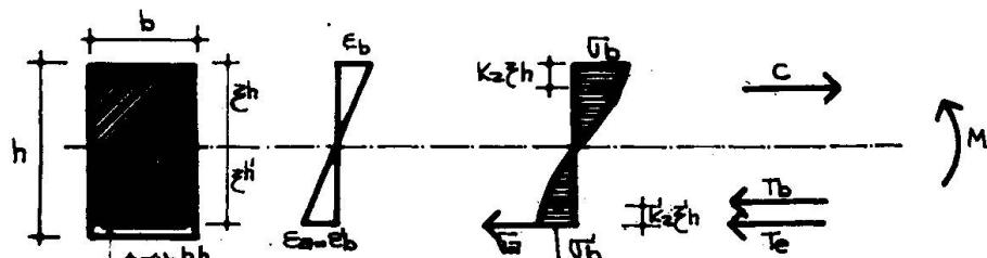
FIG. 1 STRAINS,STRESSES AND INTERNAL FORCES
