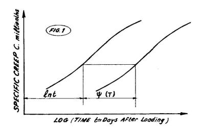
Hence knowing the specific creep curve at one temperature for T.S material one can determine the specific creep curves for that material at any other constant temperature T, by simply replacing the argument t in reference curve by  $t \not Q$  (T).
