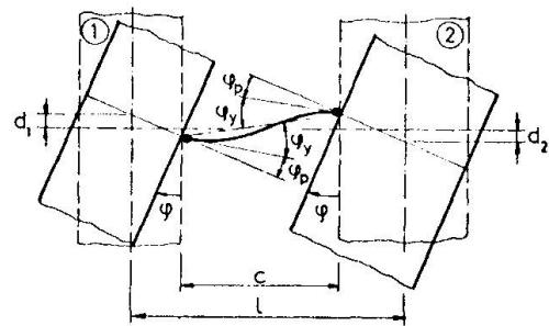
Fig. 6 Deformed position of shear wall and plastified lamina.
