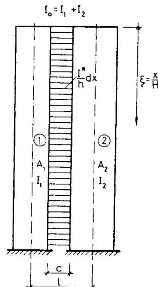
Fig. 2 Laminar model of coupled shear wall.
