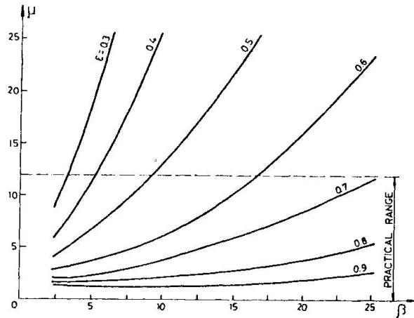
Fig. 7 Rotational ductility factor of coupling beam end.
