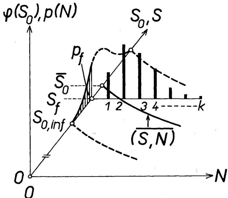
Fig.2. The broken probability distribution of the low-cyclic fatigue phenomenon
