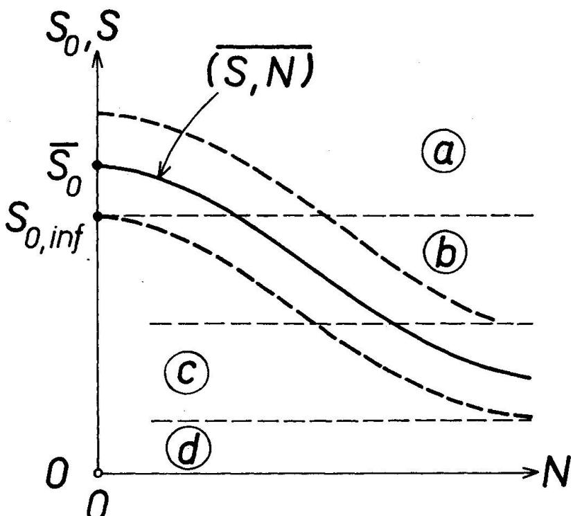
Fig. 1. Fatigue ranges: (a) low-cyclic,
