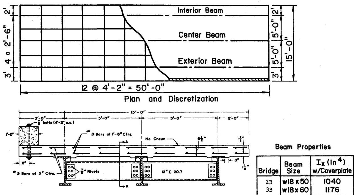
Fig. 1 Test Bridge; Left Beam = Exterior Beam,
