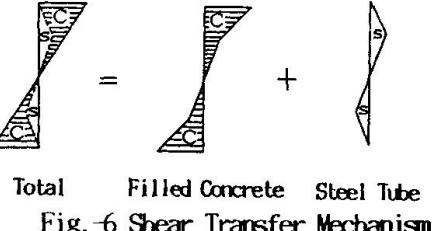
Total Filled Concrete Steel Tube
