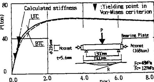
Fig. 5 Bending Test
