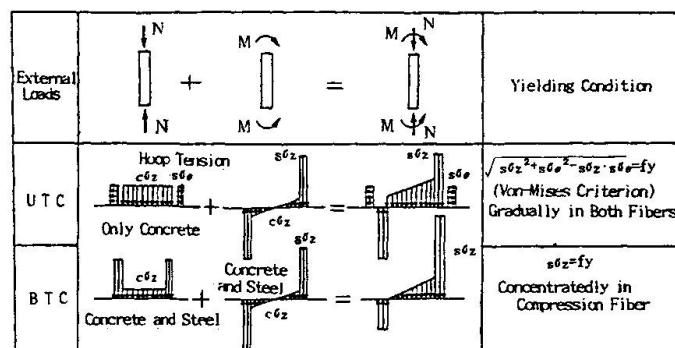
Fig.-2 Stress Condition under Combined Force
