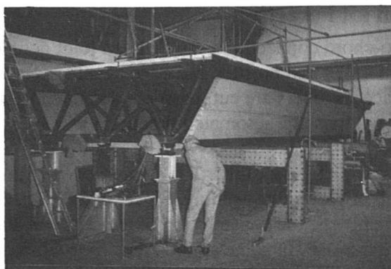
Figure 4 Cambridge half scale model of SPACES deck
