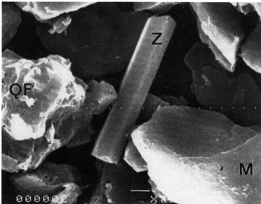
B. Detailed view of a coarse zeolite crystal (Z, authigenic?), mica flakes (M) and quartz and/or feldspar grains (QF) by SEM (core ME-68-89, sample depth 110–112 cm, 2–16 \mu\text{m} fraction). Scale bar is 1 \mu\text{m} .
