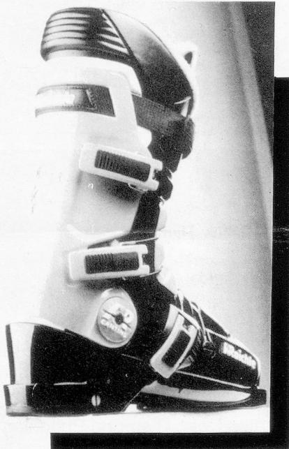
The new Ceramic-Fit-System, developed by the well-known Swiss ski-boot manufacturer Raichle, consists of an active "breathing" bubble sown into the inside of the boot. This bubble is divided into chambers and filled with microscopically small ceramic hollow spheres. The spheres immediately adapt to the individual contours of the foot inside the boot. When the boot is snapped on, the air is forced out of the ceramic bubble which
