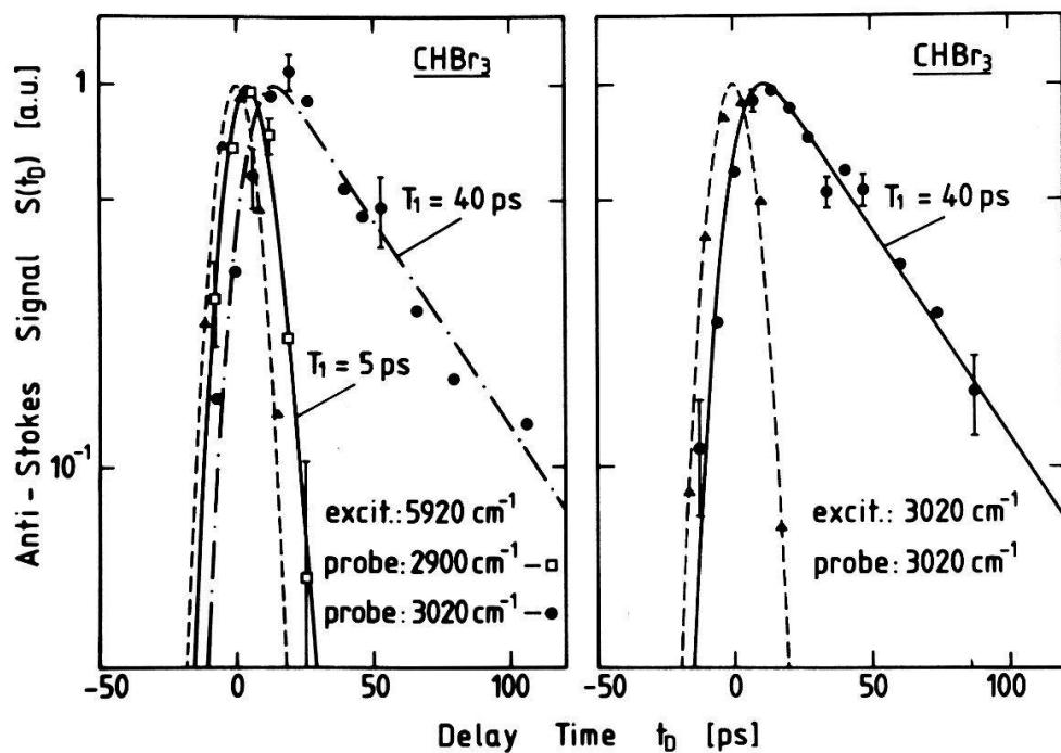
Figure 2. Spontaneous anti-Stokes probe scattering  $S(t_D)$  of the CH-stretching mode of neat  $\text{CHBr}_3$ :
