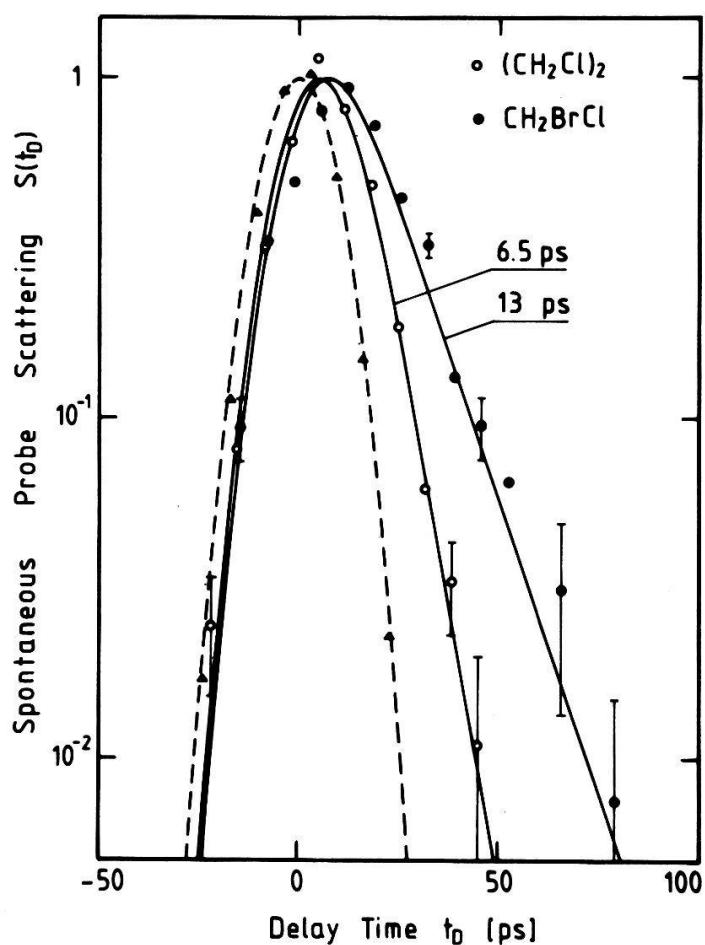
Figure 1. Spontaneous anti-Stokes scattering signal  $S(t_D)$  of the probe pulse versus delay time  $t_D$  for the symmetric  $\text{CH}_2$ -stretching modes of  $(\text{CH}_2\text{Cl})_2$  ( $\circ$ ) and  $\text{CH}_2\text{BrCl}$  ( $\bullet$ ); broken line and full triangles represent the instrumental response of the  $(\text{CH}_2\text{Cl})_2$  measurement.
