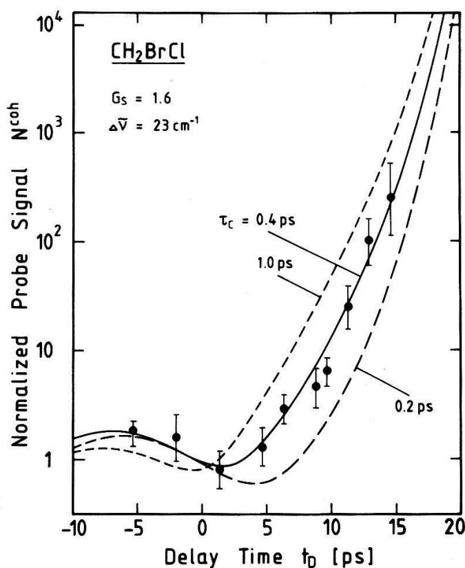
Figure 3. Normalized probe signal  $N^{coh}(t_D)$  versus delay time  $t_D$  for the  $\nu_1$ - $\text{CH}_2$ -mode of neat  $\text{CH}_2\text{BrCl}$ ; experimental points; theoretical curves
