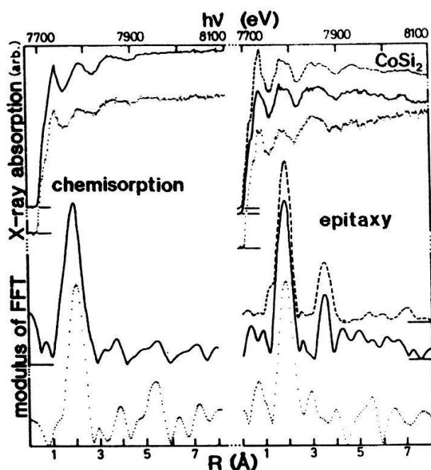
Fig. 1 Co K-edge SEXAFS spectra and modulus of Fourier transform (FFT). Left panel: chemisorption of 0.5 ML Co/Si(111) 7x7. Data and FFT for normal incidence (continuous line) and grazing incidence (dotted curves). Right panel:  $\text{CoSi}_2$  standard (dashed curves) and epitaxial 2D- $\text{CoSi}_2$ /Si(111) at normal incidence (continuous line) and grazing incidence (dotted curve).
