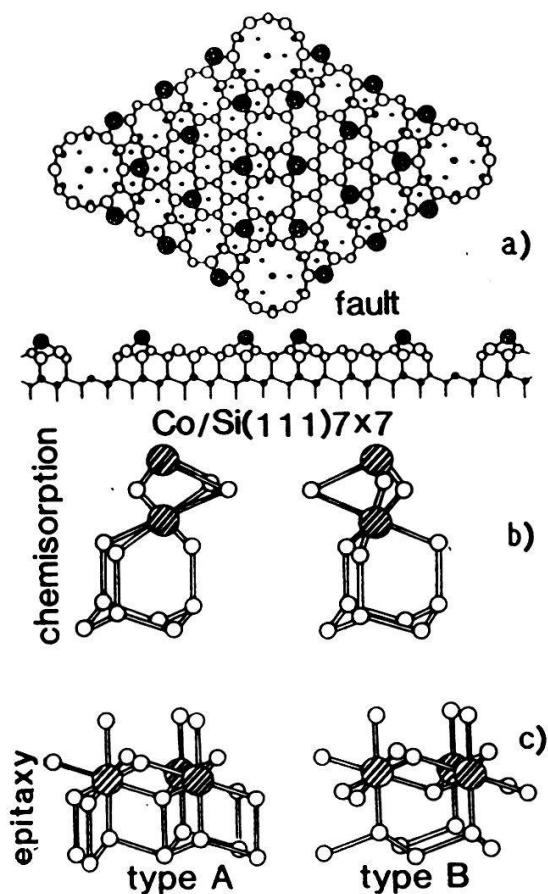
Fig.2 a) top and side view of the DAS model of Si(111)7x7. The cross hatched atoms are the Si adatoms. b) SEXAFS derived model for the chemisorption of Co (large hatched atoms) onto Si(111)7x7, both on unfaulted (left) and faulted (right) 7x7 sites. c) Hamann's models [5] of type A and B  $\text{CoSi}_2/\text{Si}(111)$  interfaces compatible with the SEXAFS results on the annealed samples.
