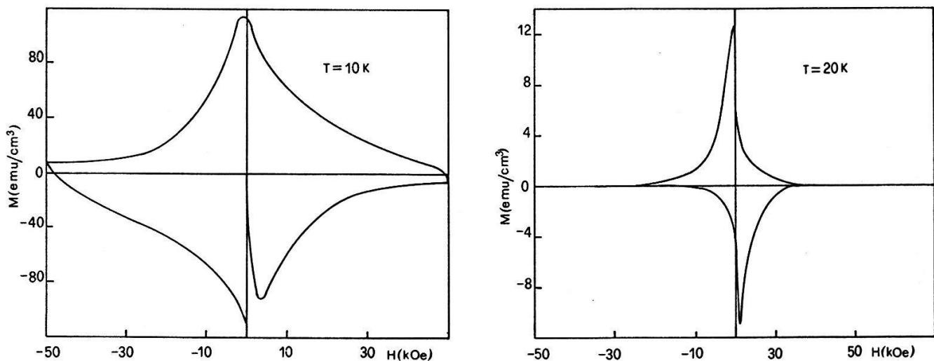
Fig. 1 Magnetization cycles
