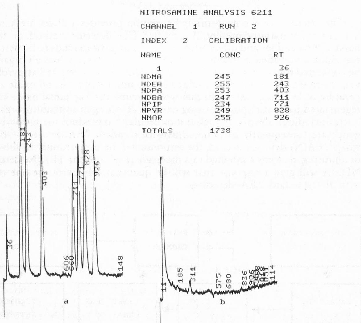
Fig. 3. a) Chromatogram of standard solution of nitrosamines
