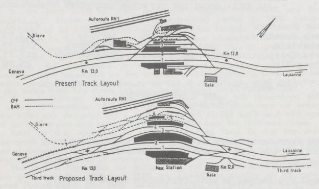
Track plan of Morges station, before and after proposed reconstruction
