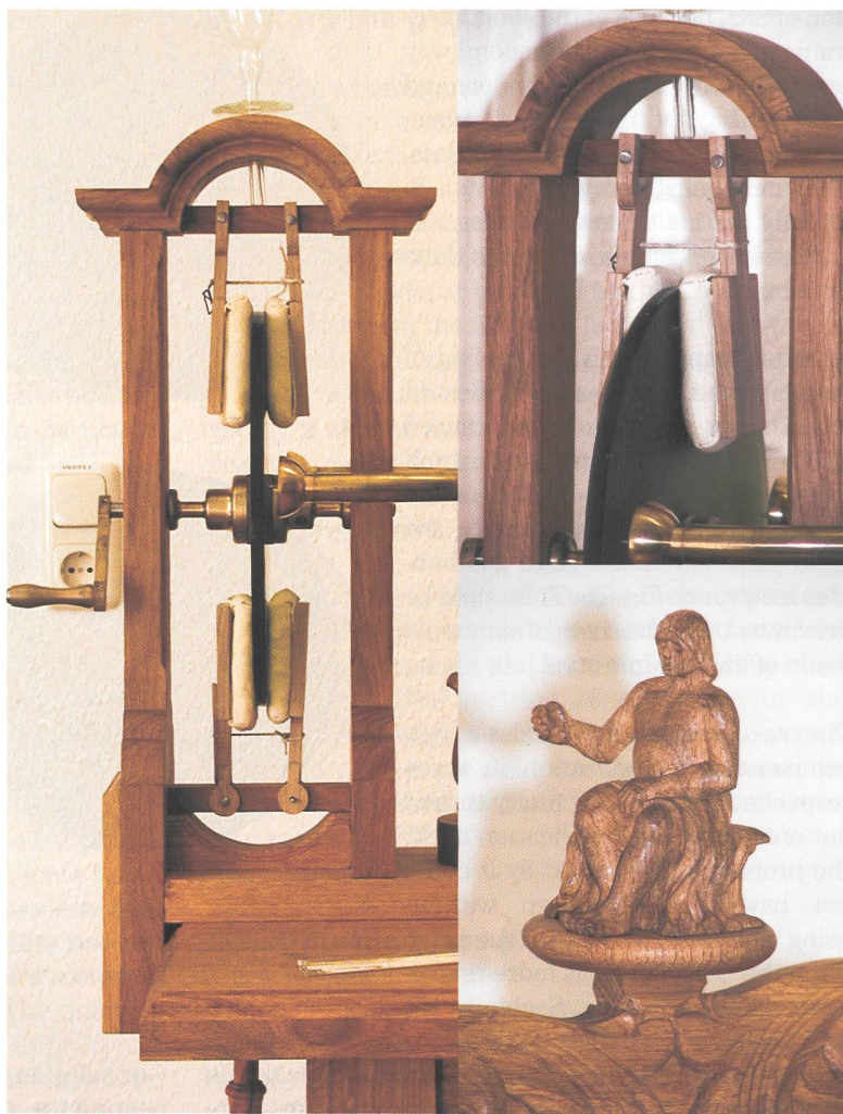
Fig. 8. Details of the replication of Schmidt's electrical machine (side view, the cushions and a carved figure of Zeus).
