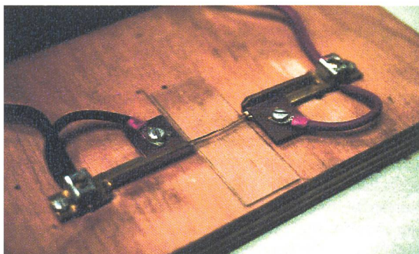
Fig. 6. Our deflagration apparatus. The gold wire (center) is mounted above a glass slide.
