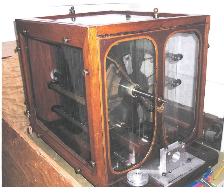
Fig. 10. The Töpler electrostatic machine used by Guye (courtesy of The Geneva Science Museum).
