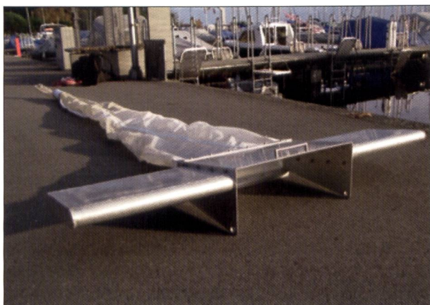
Fig. 1. The Manta trawl used to sample microplastics. Equipped with a 300 µm sieve, its mouth is 60 cm wide and dips 25 cm into the water. Picture: Vasco Neuhaus.
