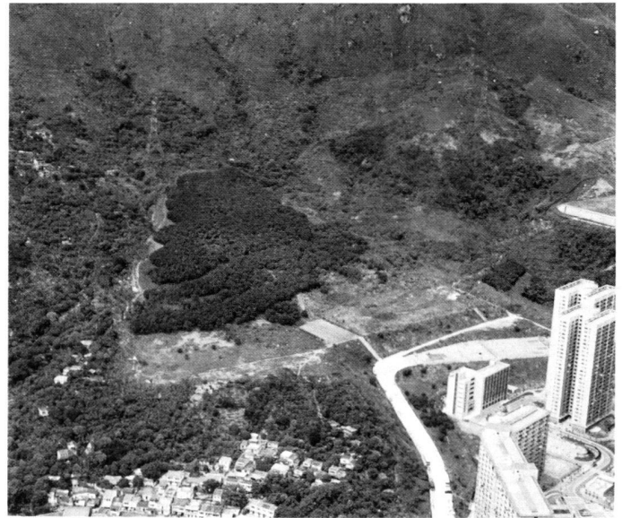
Left: Castle Peak. The reformed slope in 1980 after grassing. Eroded crests in the distance. Photo: Survey Division Hong Kong Government
