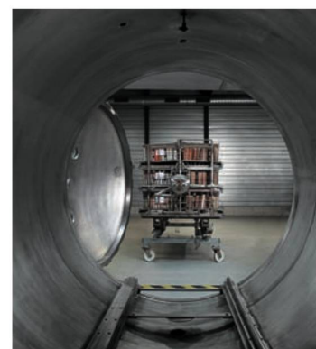
Papersave swiss plant, Wimmis. A “charge” awaits deacidification.
