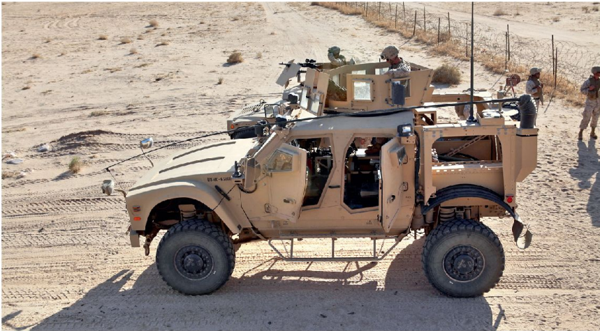
Ein M-ATV (mine-resistant, ambush-protected all-terrain vehicle) des United States Marine Corps. Bild: U.S. Marine Corps
