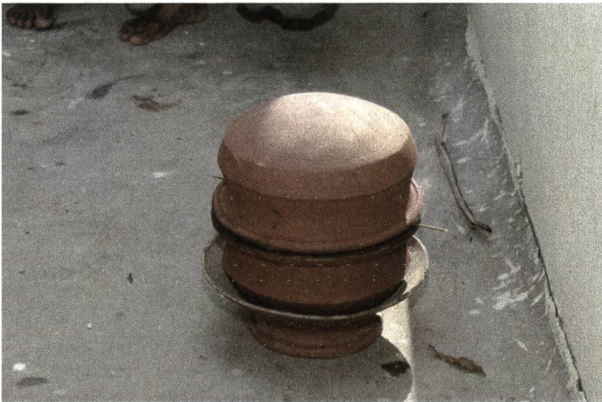
Figure 5: Closing the pot for the process of sublimation.
