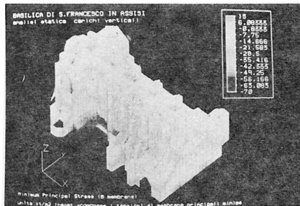
Pic.16: Damages in the Giotto frescos Pic.17: Mathematical models of Basilica of St. Francis in Assisi
