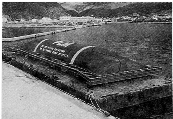
Fig.4 Flexible-mound during airtightness test on a barge (40m(L) x 9m(W) x 3m(H))
