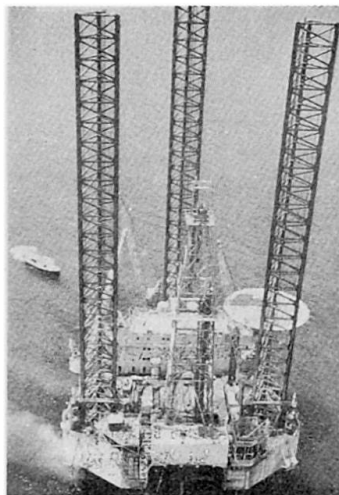
Fig. 6 Self-raising platform, "TRIGONE"
